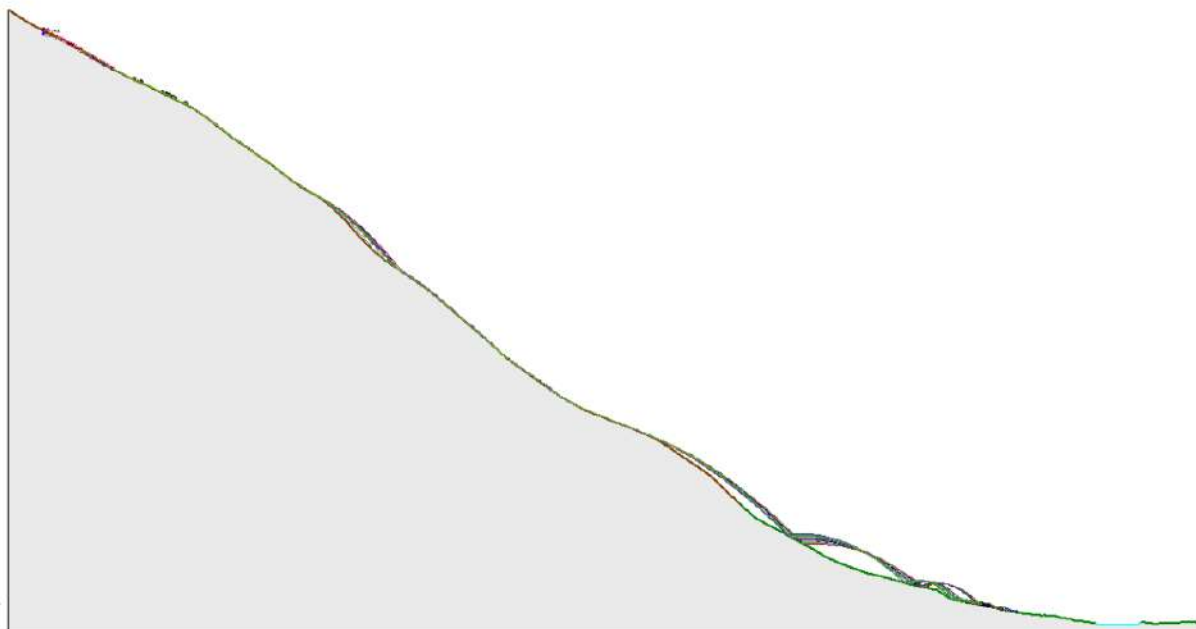
Fig. 8-11: Simulation result of M-D6 t_2 without placing a rockfall barrier.
