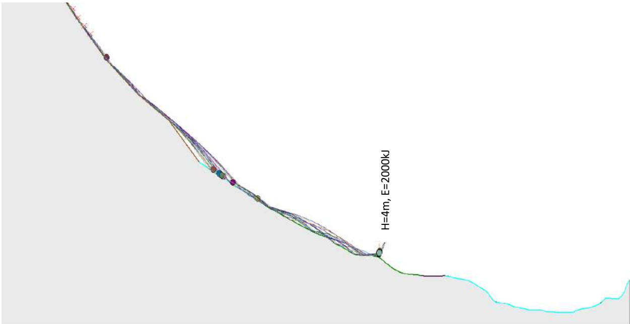
Fig. 8-5: Visualisation of the simulation result of M-D4 t_1 with placing a rockfall barrier in front of the road.
