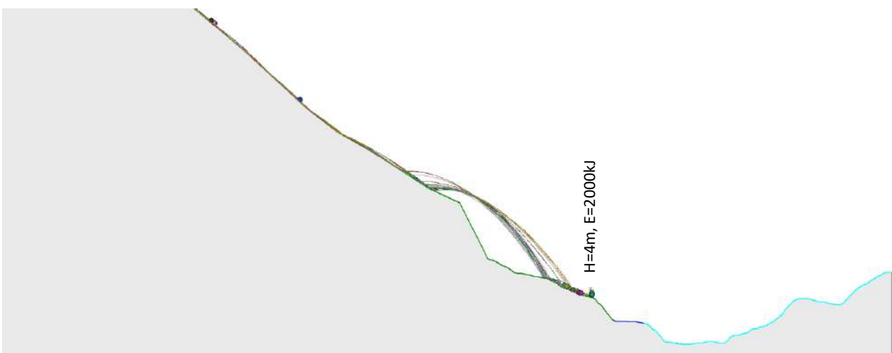
Fig. 8-7: Visualisation of the simulation result of M-D4 t_2 with placing a rockfall barrier in front of the road.
